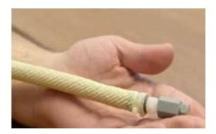
Figure 1.1. Fiber Reinforced Elastomeric Enclosure (FREE)
