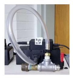
Figure 5.9. TR pressure regulator with closed outlet
