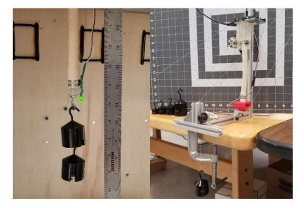
Figure 6.6. Axial and torsional loading of a FREE
