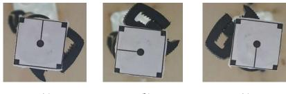
(a) (b) (c) Figure 4.10. Images of the FREE end cap at (a) 0 psi, (b) 5 psi, and (c) 8.7 psi
